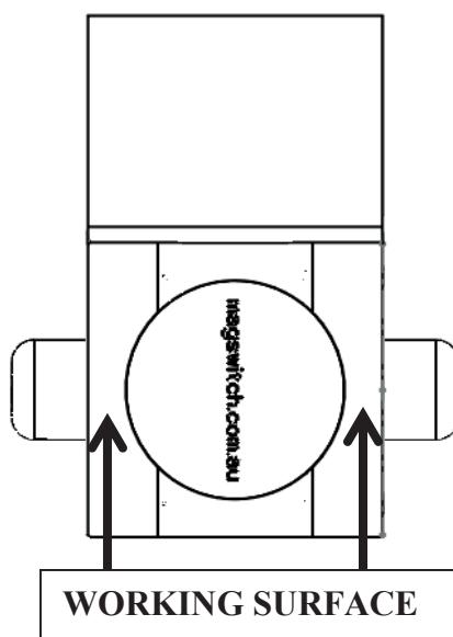
\* Max Breakaway determined in laboratory environment on 2" thick SAE1018 Steel with surface roughness 63 micro inches. Many factors contribute to the actual breakaway force in each application. Always test the magswitch in each application before deployment. Refer to the magswitch information booklet for more information.
