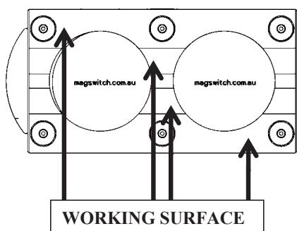
\* Max Breakaway determined in laboratory environment on 2" thick SAE1018 Steel with surface roughness 63 micro inches. Many factors contribute to the actual breakaway force in each application. Always test the magswitch in each application before deployment. Refer to the magswitch information booklet for more information.
