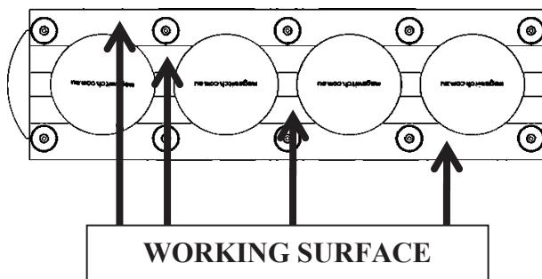
\* Max Breakaway determined in laboratory environment on 2" thick SAE1018 Steel with surface roughness 63 micro inches. Many factors contribute to the actual breakaway force in each application. Always test the magswitch in each application before deployment. Refer to the magswitch information booklet for more information.
