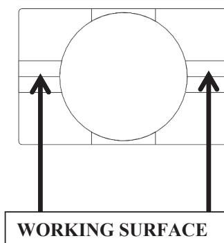
\* Max Breakaway determined in laboratory environment on 2" thick SAE1018 Steel with surface roughness 63 micro inches. Many factors contribute to the actual breakaway force in each application. Always test the magswitch in each application before deployment. Refer to the magswitch information booklet for more information.
