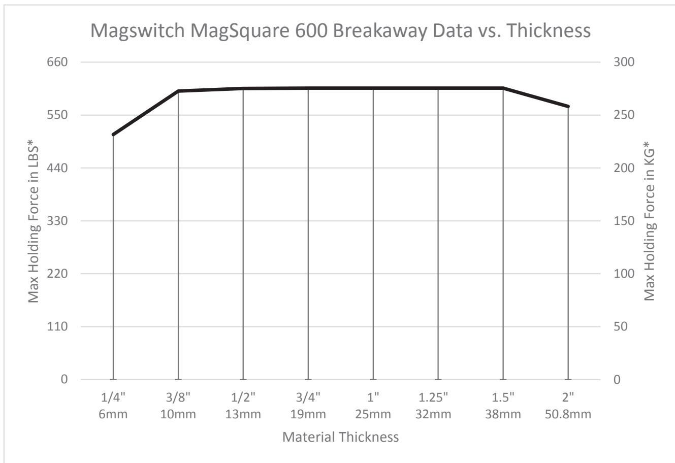
\* Max Breakaway determined in laboratory environment on 2" thick SAE1018 Steel with surface roughness 63 micro inches. Many factors contribute to the actual breakaway force in each application. Always test the magswitch in each application before deployment. Refer to the magswitch information booklet for more information.
