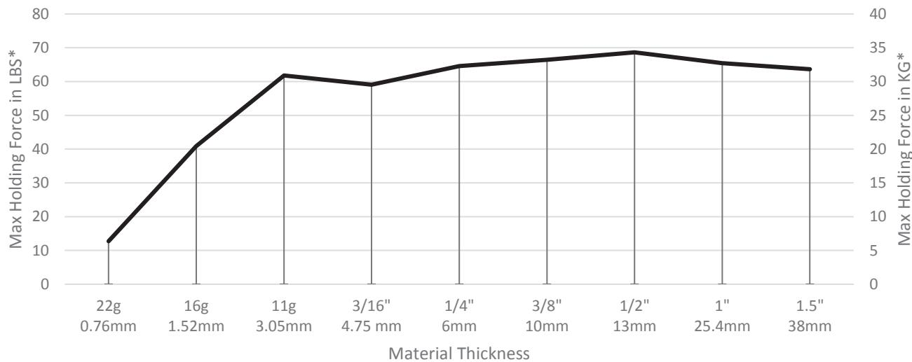
\* Max Breakaway determined in laboratory environment on 2" thick SAE1018 Steel with surface roughness 63 micro inches. Many factors contribute to the actual breakaway force in each application. Always test the magswitch in each application before deployment. Refer to the magswitch information booklet for more information.
